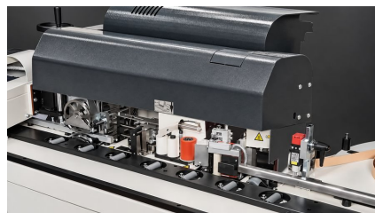
WORKING UNITS UNDER THE HOOD: EDGE FEED, GLUE ROLLER, PRESSURE ROLLERS AND END TRIMMING
