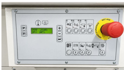
TEMPERATURE DISPLAY, UNIT SELECTION WITH LED BUTTONS AND EMERGENCY STOP
